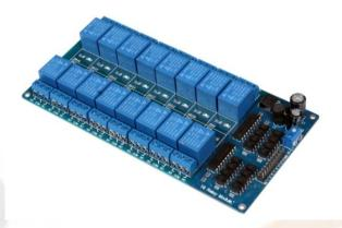
This is a 12V 16 Channel Relay Module with Light Coupling LM2576 Power Supply, Be able to control various appliances and other equipment with a large current. It can be controlled directly by Micro-controller (Arduino, 8051, AVR, PIC, DSP, ARM, MSP430, TTL logic).
